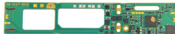
Typical „Individual” decoder; for a Fleischmann SBB Ae 6/6 (a sound decoder directly integrated in the loco board, components used similar to the standard type MX649)
