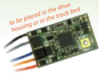
MX820E standard layout, one-sided board assembly
