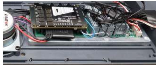
Märklin-LGB G scale „Allegra“ (RhB ABe) after installing supercap energy storage, speaker, and decoder MX695LS.
